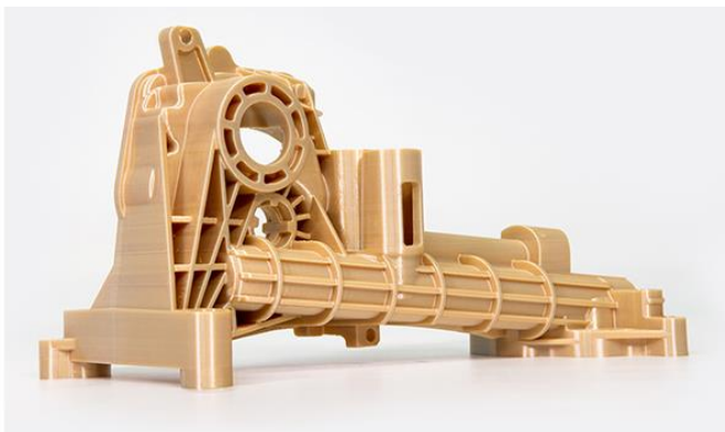
Part printed with SABIC's ULTEM™ AM9085F filament after AMS31F support material is removed
