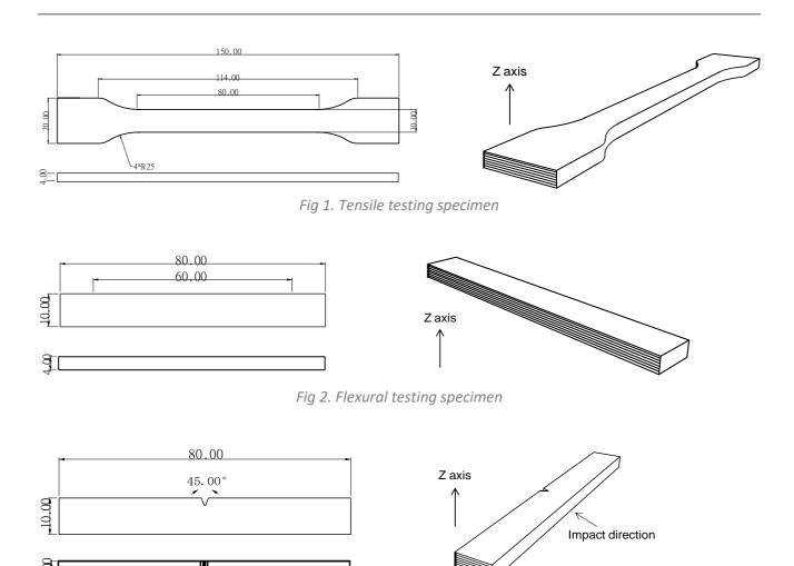
Fig 3. Impact testing specimen
