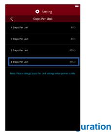
The stepper driver needs to be adjusted because we have changed the previous motor(s) to smaller one(s) that requires a lower current. There is a risk that the motors will overheat and cause damage if they are not adjusted.
