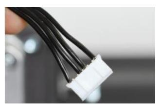
To reverse the two cables, you can use a sharp tool to lift the little plastic tab on the connector and gently pull the crimping contact out of the housing with your hand.
