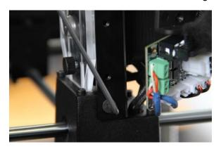
3.2 Remove the 2 screws on the back side with 2.5mm hex wrench.
