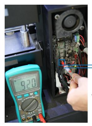
Turn the adjusting screw carefully until you reach the value of about 0,9V(900mV), clockwise increase, counter-clockwise decrease.
