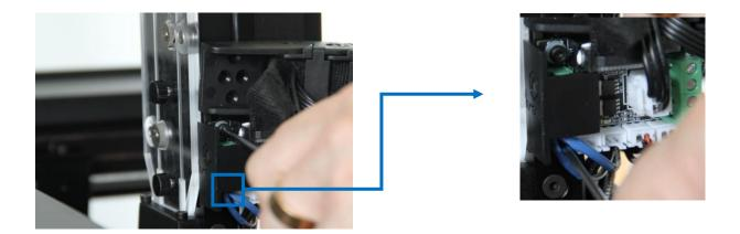
3.5 Remove the original extruder by pulling it straight up.
