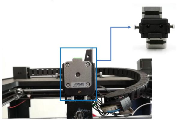
4.2 Install the original screws to the left and right (2,5mm hex wrench). Do not tighten the screws fully.
