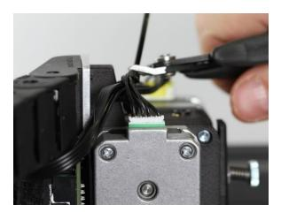
6.5 Do the same operation at the bottom and cut of the ends.
