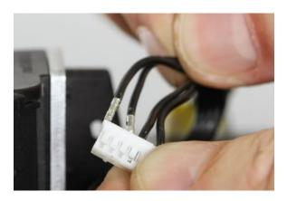
6.2 Change positions of those two cables by pushing it back into place. Reverse position 1 and 3.
