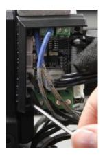
5.3 Fix the cable chain with the original screws.
