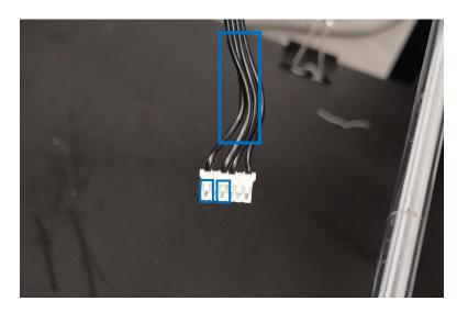
6.3 Plug the unmarked cable onto the rear motor and the marked cable into the front motor.
