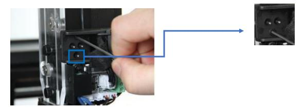
3.4 Remove the 2 screws fixing the extruder board and its origin cover with a 2.5mm hex wrench.
