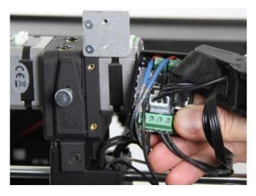
5.2 Attach the board holder. Note that the bottom screw is M2.5 and the upper one is M3.
