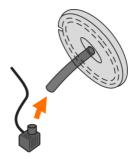
4. Connect the Pump to the other end of the Water Tube, aligning the Power Cord in the same direction as the slot in the Screen Cover.
