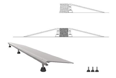
• Adjust the length of the adjustment feet to the desired wedge height
