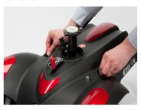
2. Connect the battery pack. Refit the shroud and tighten the two knobs to secure.
