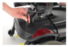
8. Plug the cable from the joystick remote into the port at the centre of the powerchair base.
