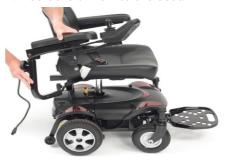
5. Set the arms to the required width then secure by turning the armrest knobs clockwise.
