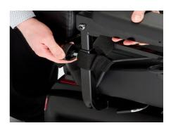
6. Affix the headrest to the top of the seat by inserting the headrest posts into the holes in the top of the seat.
