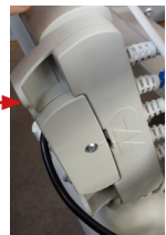
Cable cover unclips/clips into place
