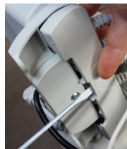
Cable cover unclips/clips into place
