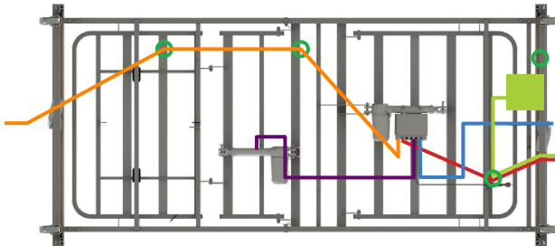
8.4.1 Bed cable routing
