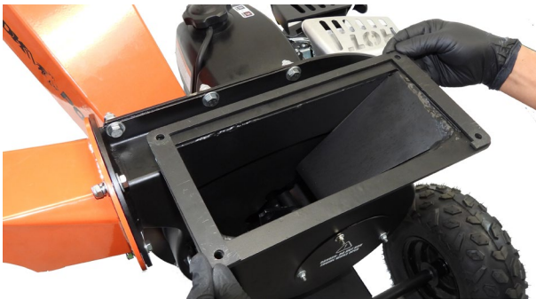
3. Align holes and Door Frame
