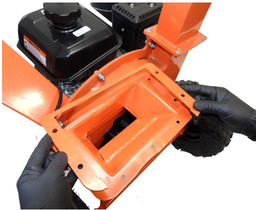
3. Align holes and Door Frame
