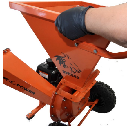
2. Remove chute and Clean the mounting area of all debris
