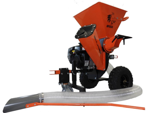
4. Run on high RPM with slide door Closed to operate the Vacuum.
