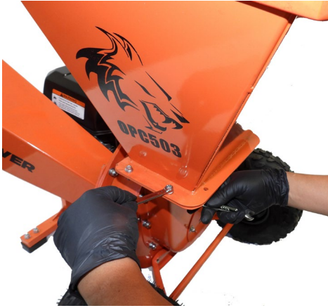
1. Remove bolts and Feed Chute
