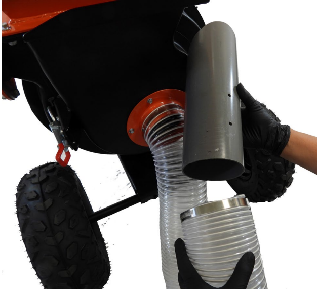
1. Attach Nozzle with Hose Clamp
