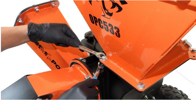
1. Remove bolts and Feed Chute
