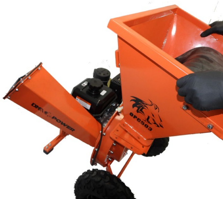
5. Remount the feed chute and bolts
