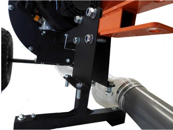
1. Bolt wheel mounts to tow bar
