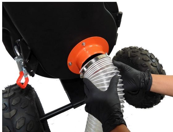
5. Install Hose and Hose clamp
