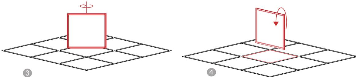
3. Aligning the site of panel light and ceiling board and finish the installation. (Picture 5, 6)
