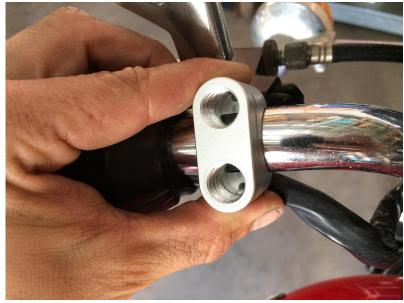
3.Centre punch marked holes and drill 6mm to 10mm depending on your wiring need. Taking care to be  $90^{\circ}$  to the face being drilled.
