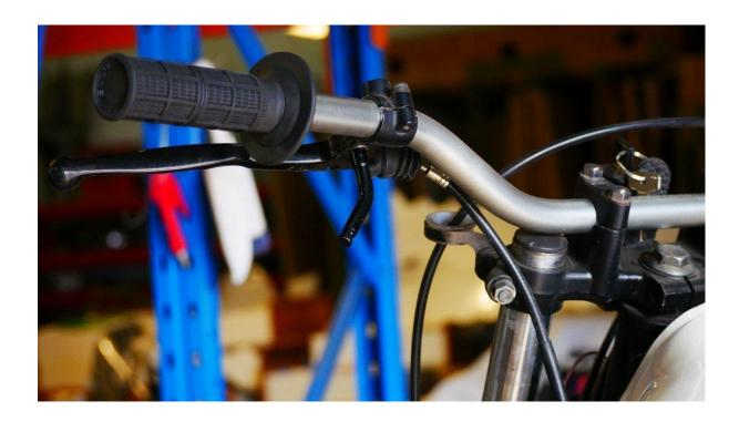
3. Using some locktite, thread the second M6 nut onto the exposed thread from your mirror kit, then thread on the mirror arm.
