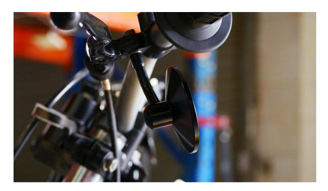
5. **Double check the steering stops** to make sure nothing is fouling your movement, adjust the mirror to suit, then get out riding!
