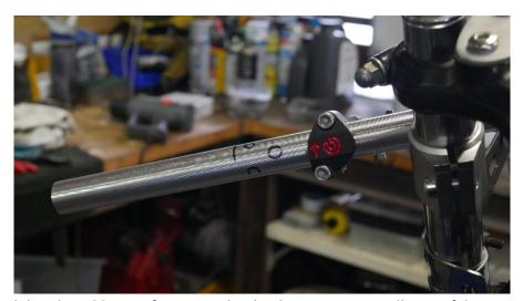
5. It is reccomended that the soldering of your switches be done prior to installation of the wiring, using a low heat soldering iron and holding the pushbutton in a vice. Too much heat can cause damage to the switch internals and limit switch life. Use enough cable to reach the termination point and limit joins.
