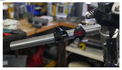
4 .Centre punch marked holes and drill 6mm to 10mm depending on your wiring needs. Taking care to be  $90^{\circ}$  to the face being drilled.
