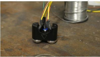
8. Run wiring internally through handlebar, taking care of any sharp edges.
