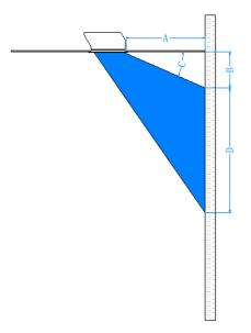
Step 2. Ceiling opening: The product needs a 285mm\*585mm ceiling opening. Drill the opening at the installation positions calculated in step 1.
