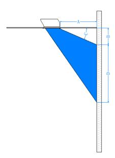
Step 2. Ceiling opening: The product needs a 1135mm\*125mm ceiling opening. Drill the opening at the installation positions calculated in step 1.
