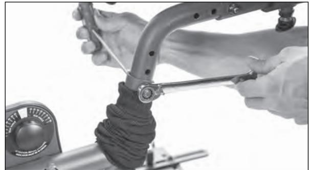
2. Use a hex wrench and 13mm wrench and remove nut and washer.
