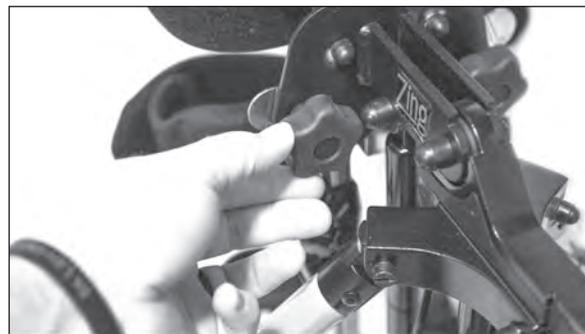
Abduct each leg out to the desired position up to 15 degrees per leg. Tighten securely
