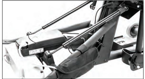
⚠ **Caution:** Ensure the cables are attached properly per the instructions for use. Do not allow the cables to drag on the floor or to catch on objects. A pouch is installed at the rear frame to store the power cord when not in use.
