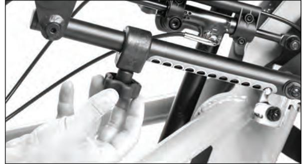
**Adjusting to a shorter setting:** Adjust the following arm (back angle) first by depressing the spring button and moving no more than two holes at a time. Then adjust the seat tube (seat depth) one hole at a time. Continue this sequence until you achieve the desired setting and the colors on the seat tube and following arm match.
