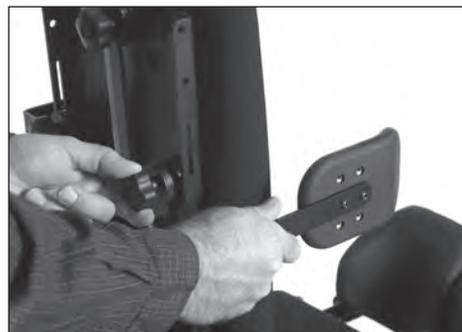
The lateral supports have a number of attachment holes on the back of the pad allowing for additional positions vertically and horizontally. The pads can also be bolted on at a straight, 90°, 180°, or 270° position.
