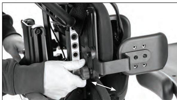
To adjust the lateral support height, loosen knob, adjust to desired position. Tighten securely.
