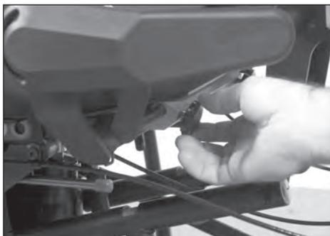
The hip supports have a number of attachment holes on the back of the pad allowing for additional positions vertically and horizontally. The pads can also be bolted on at a straight, 90°, 180° or 270° position.
