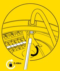
Screw the wiring cover to the base plate.
