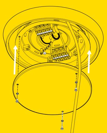
Fit the face plate, ensuring all cables are aligned through the circular slot. The magnets already attached to the face plate will hold it in position.
