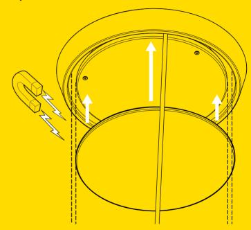
Raise shade above lampholder to enable easier fitting of the LED lamp.
