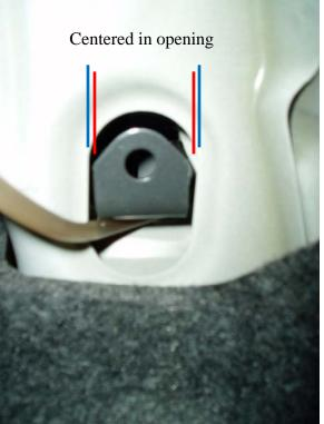
7. Install the Oswald Performance bottom mount using the factory bolts from the vertical bars.
