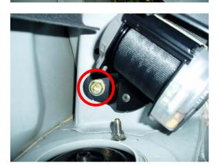
5. Remove the three nuts on each strut top.
