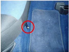
2. Remove seat back by removing the three bolts (left, right, and center).
