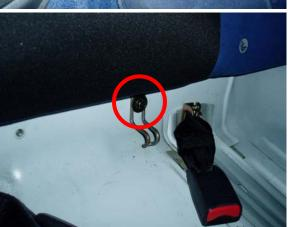
3. Remove the two vertical bars (left and right) by removing the four bolts each (two at the top and two at the bottom). Remove the trunk trim panel by removing the four plastic clips (circled).
