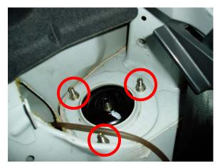
6. Install the Oswald Performance strut tops on each side using the factory nuts. The left and right strut tops are different and will only fit on their respective sides. Be careful tightening the nuts as the studs are notorious for breaking. As you tighten the nuts try to keep the strut top centered in the bulkhead opening.
