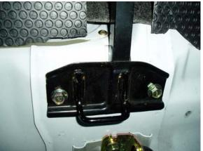
4. Remove the two side seatbelts by removing the bolt shown.
