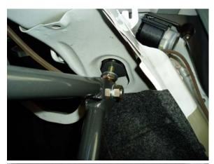
10. Insert the large bolt with washers through the brace and bottom mount as shown. Thread the large locknut on but leave it loose so that the brace is free to move up and down.
