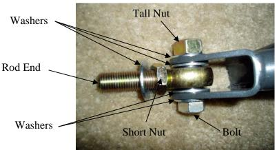
9. Slide the rod ends into the strut tops.
