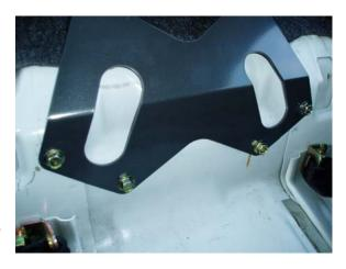
8. Prepare the Oswald Performance brace by installing the two rod ends (one on each side) as shown. Thread the short jam nuts all the way down on the rod ends.
