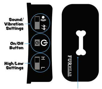
The bone shaped LED light will shine green when it is turned ON and red when it is turned OFF. LED light will flash red when the battery is at 10% or less.
