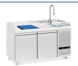
The P3 is the ultimate refrigerated prep table. Its worktop is a true masterpiece, fitted with four side-mounted nozzles, a recessed bottom sloping down to the sink, a polyethylene chopping board, a perforated stainless steel tray and a mixer tap with pull-out spray. Monocoque food-grade stainless steel construction with an operating temperature of -2 °C +2 °C. Supplied with natural R290 refrigerant and 4x 40x60 cm fish trays per door.
