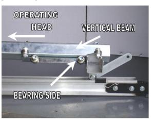
• Now connect the slide unit to the garage door motor traveller by using the link.
