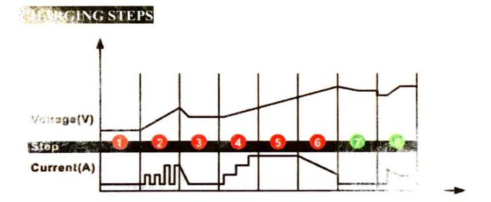
STEP 1: DIAGNOSIS (Check if battery has connected with the charge check battery voltage)
