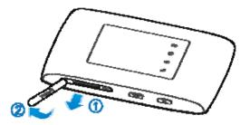
2. Install a micro-SIM card to the micro-SIM card slot.
