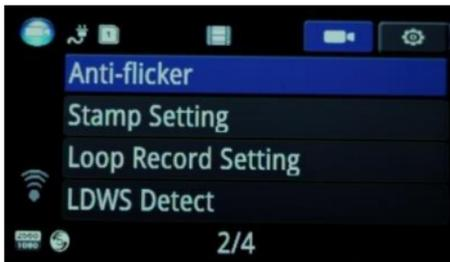
**Frequency:** Three modes: Auto/60Hz/50 Hz , the default is 50 Hz
