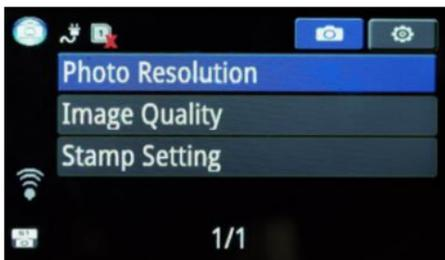
**Photo resolution:** Three modes:4M(2688×1512 16:9)/9M(4000×2250 16:9)/13M(4800×2700 16:9) the default is 4M
