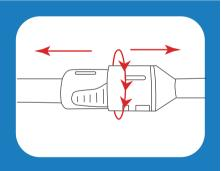
Turn the valve backward to disconnect the pump.
