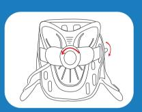
① Turn the back knob counter clockwise to the loosest setting. Turn the side knobs backwards to loosen to the loosest setting.
