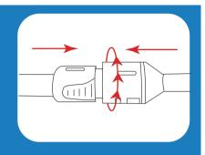
⑤ Connect the pump to the valve, hold and turn the pump side valve forward to lock.
