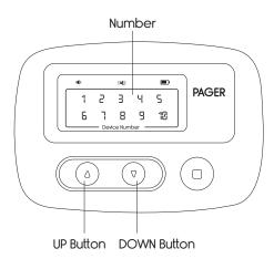
**Step 3:** There are 10 channels on the pager for programming up to 10 individual wireless devices. Select a number for programming by pressing the UP or DOWN arrow on the front of the pager.
