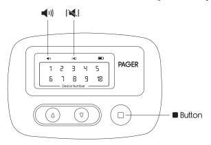
To select another notification mode, press and release the UP Button or DOWN Button on the front of the WPG. The next notification light [14] will start blinking. Continue to press and release the Up or Down buttons until the desired notification light is selected. Once you've landed on your desired notification light, press and release the Button, you will hear a 1 second beep and/ or feel a 1 second vibration. This means the current notification mode is recorded to the WPG.
