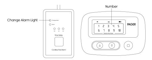
**Step 5:** The pager will beep to signal a successful connection. Then it will re-enter programming mode in case you need to connect other wireless devices. If you do not need to connect more devices press and hold both the UP and DOWN arrows on the front of the pager to exit programming mode.
