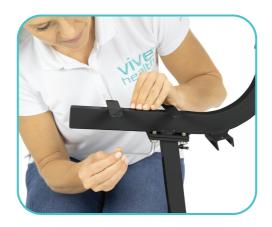
8. Position the Seat Pad and Backrest Pad on the Seat Frame and secure each in place using four (4) Frame Allen Bolts and Flat Washers. Make sure to place the washer between the bolt head and the pad bracket on the Seat Frame.
