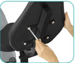
9. Position the Seat Handlebar into the square bracket on the underside of the Seat Frame and secure it in place using two (2) Handlebar Carriage Bolts, Flat Washers, and Cap Nuts. Make sure the Handlebar is fitted with the metal heart rate sensors facing up.
