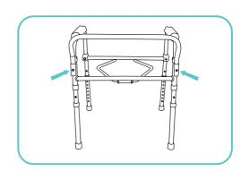
Attach the toilet seat (E) and cover (F)to the back of the frame. The toilet seat hooks should fit inside the hooks of the cover.
