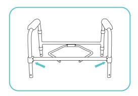
3. Turn frame upside–down. Adjust the length of the preinstalled legs (C) by pressing the rounded brass locking pin in and pushing/pulling the leg to the desired length. The locking pins will click into place when aligned with an adjustment hole.
