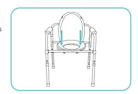
6. Lower splash guard (H) and commode bucket (G) into frame and return seat to down position. Now your seat is fully assembled.
