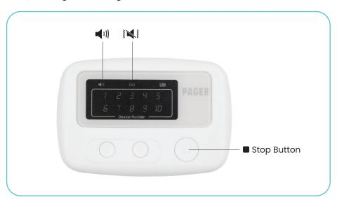
To select another notification mode, press and release the UP Button or DOWN Button on the front of the pager. The next notification light \( \) will start blinking. Continue to press and release the Up or Down buttons until the desired notification light is selected. Once you've landed on your desired notification light, press and release the Button, you will hear a 1 second beep and/or feel a 1 second vibration. This means the current notification mode is recorded to the pager.
