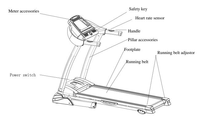
Diagram 1: T430 Motorized Treadmill
