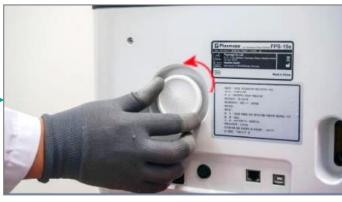
2. Remove the old HEPA filter by turning counterclockwise
