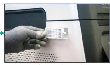
3. Remove the Ozone filter and replace it with new Ozone filter
