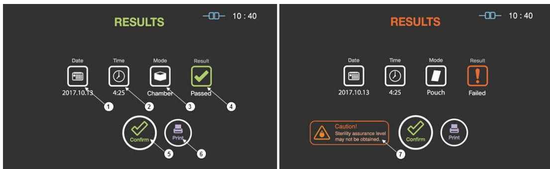
Fig. 7.1 Screens for cycle report; succeed (left) and fail (right)
