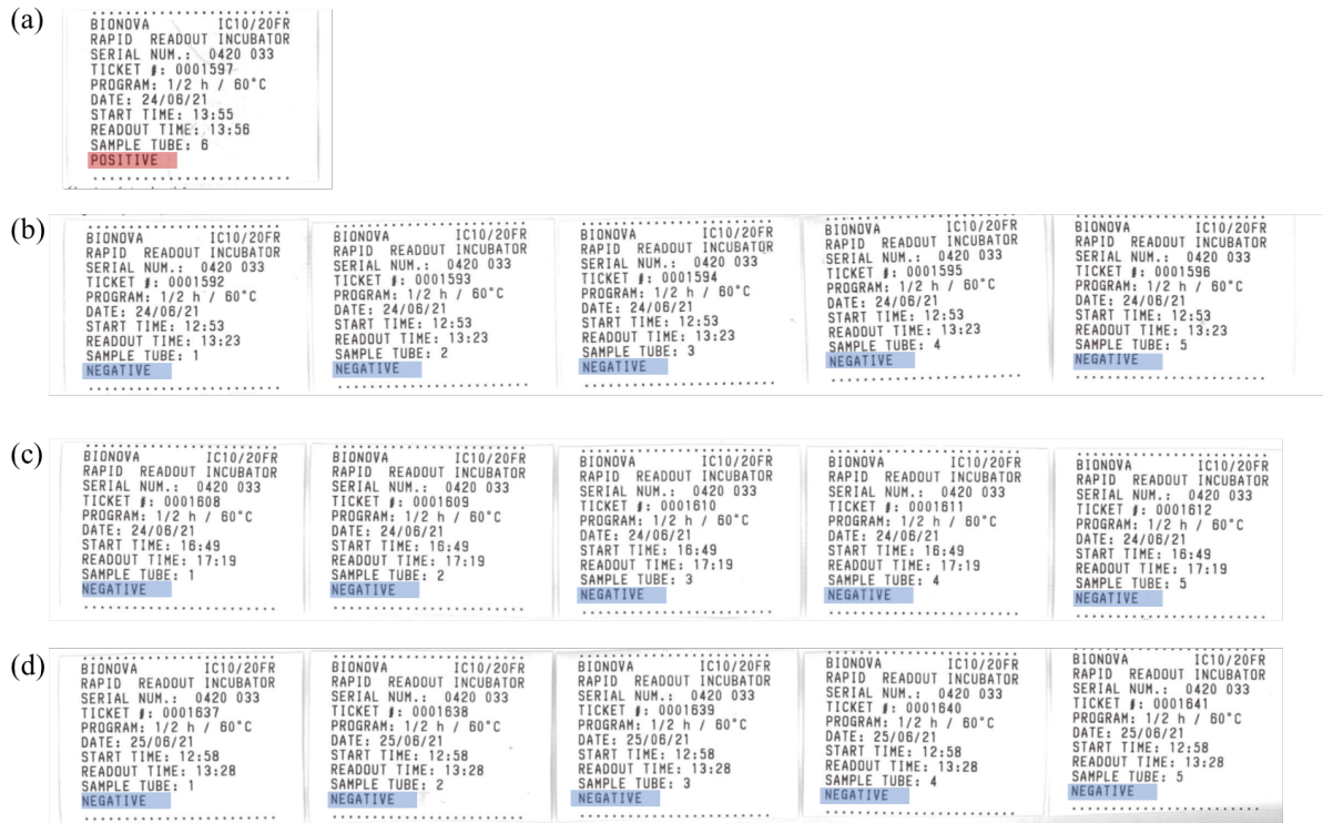
Figure 4.1 The incubation results of (a) the control and (b-d) three consecutive lumen sterilization tests for chamber mode sterilization. The negative result implies complete sterilization.
