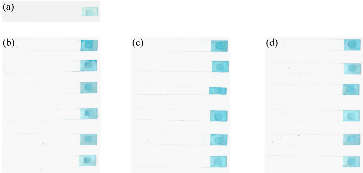
Figure 2.1 Color change result of hydrogen peroxide strip in (a) negative control and (b-d) three validation tests. It is a test sample aeration for 0, 10, 30, 60, 120, and 300 seconds in order from the top in each validation test figure.
