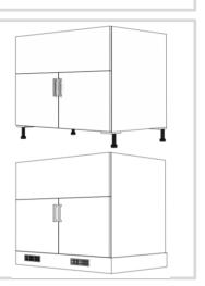
**ASSEMBLY:** WeatherStrong cabinets are built with precision dowel alignment and a fast cure solvent-free structural marine adhesive system that provides excellent flexibility. toughness and bond strength.
