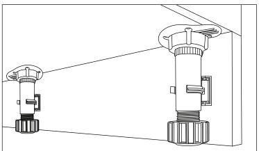
If applying toe kick around corners, adjacent panels will clip to the same corner leg. Be sure to stagger the clip plate heights so they overlay properly.
