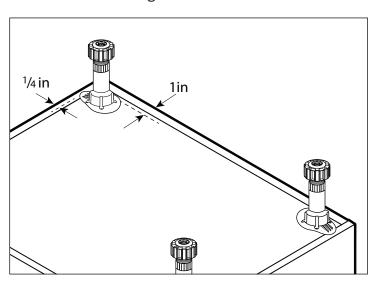
Use a phillips bit to attach the legs with the stainless steel screws supplied. DO NOT OVERTIGHTEN!
