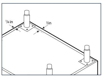
4. Adjust the leveling legs up or down to bring the cabinet to a level plumb position.
