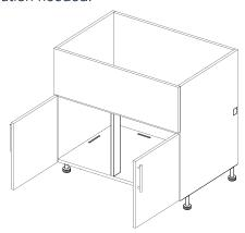
Grill Base and Side Burner cabinets will come with precut vent holes in the sidewalls and precut slots in the cabinet. There will also be precut slots in the toe kick material. This will enable any excess gas to vent from inside the cabinets. If using toe kick with your cabinets to cover the leveling legs, a piece of toe kick with vent slots has been included with your Grill Base or Side Burner cabinet.
