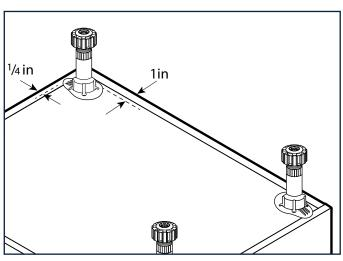
4. Adjust the leveling legs up or down to bring the cabinet to a level plumb position. Use of the longer stems may be needed in this application.
