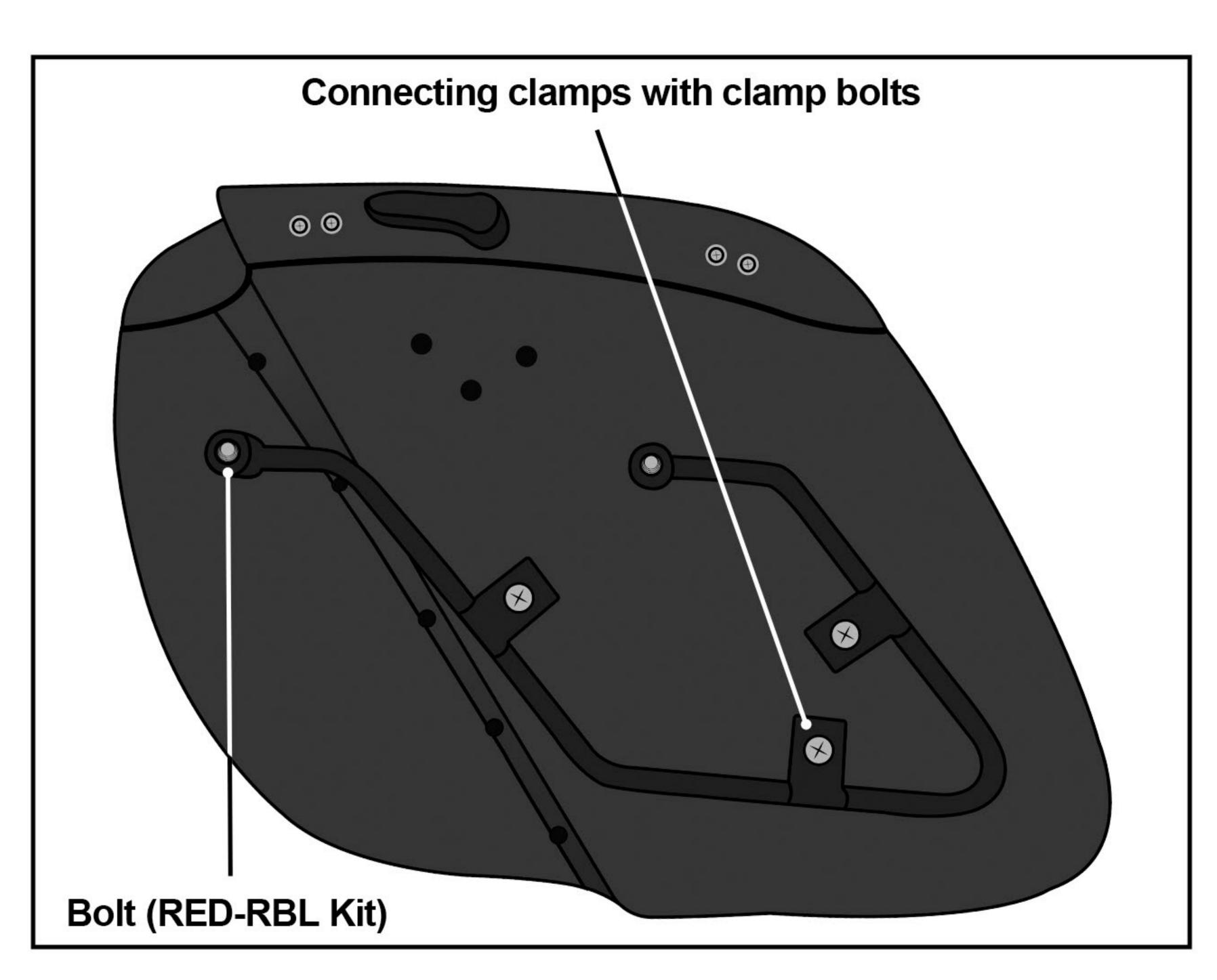
Fig 4. Attach the bag to the bracket using clamp bolts
