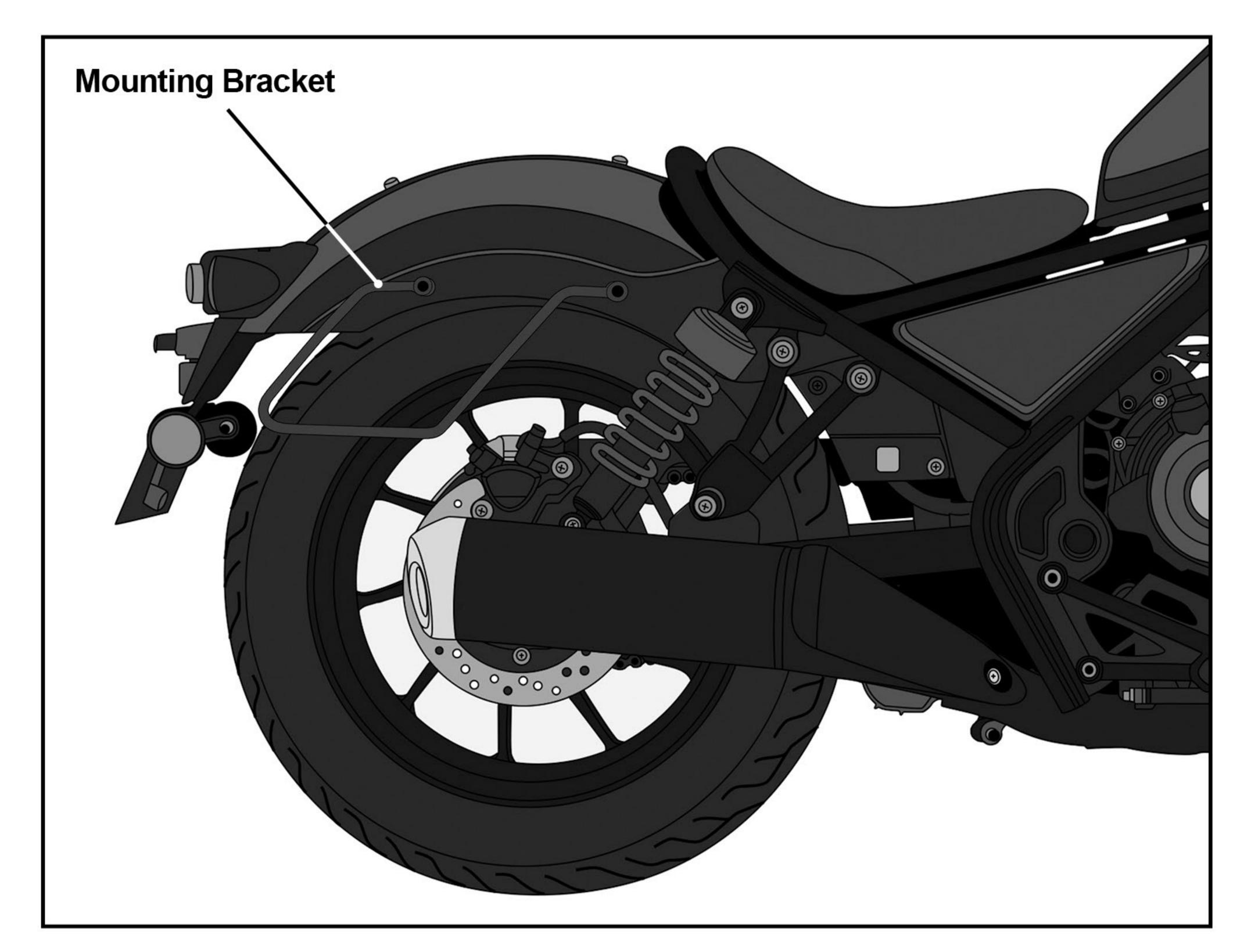
Fig 2. Install the bracket on the bag
