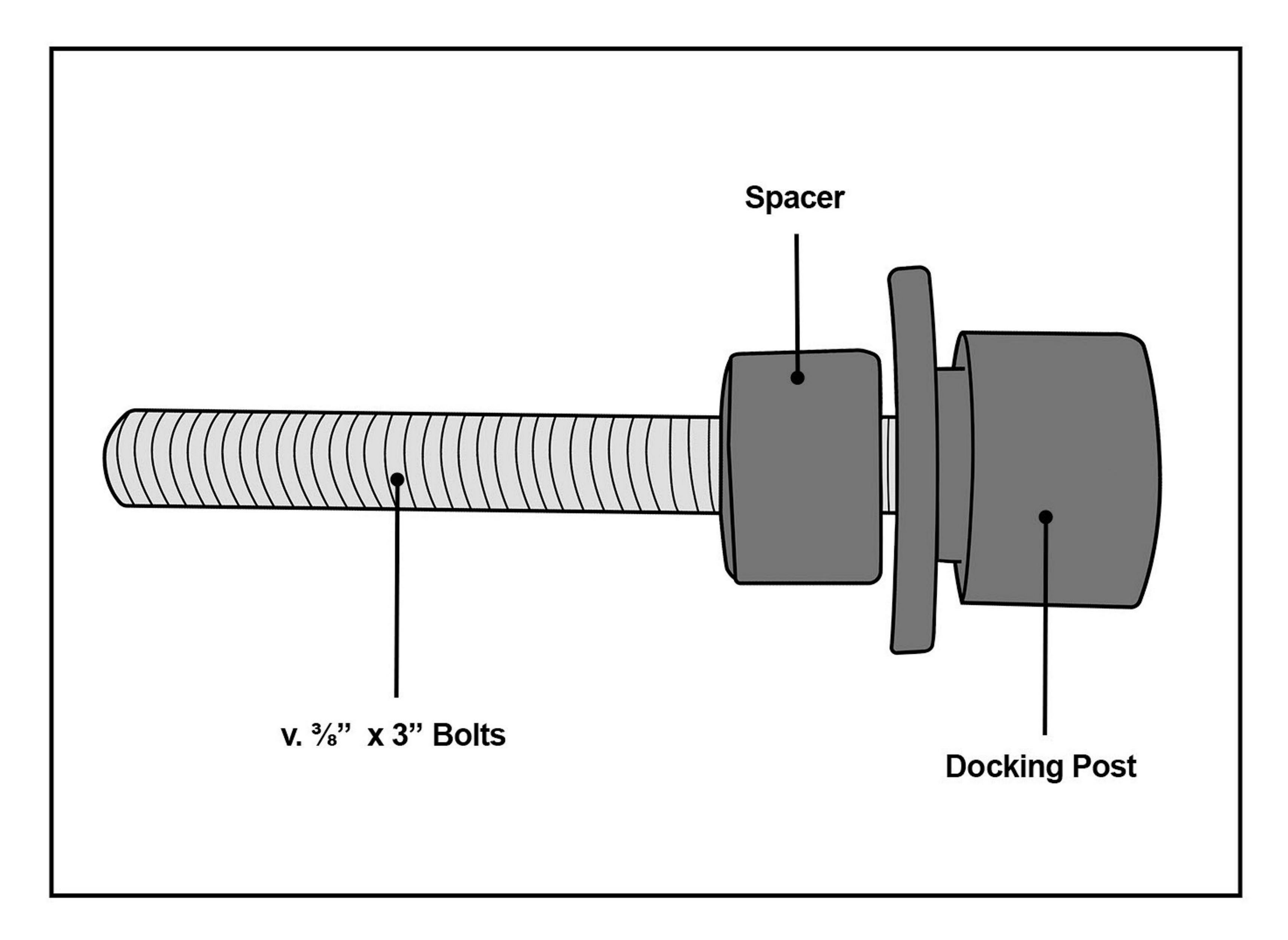
Fig 1. Bolt configuration
