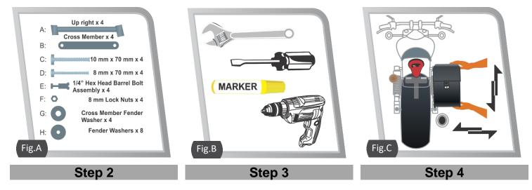
Use a marker or paint to mark the position of the fender bolts onto the back of the bag.
