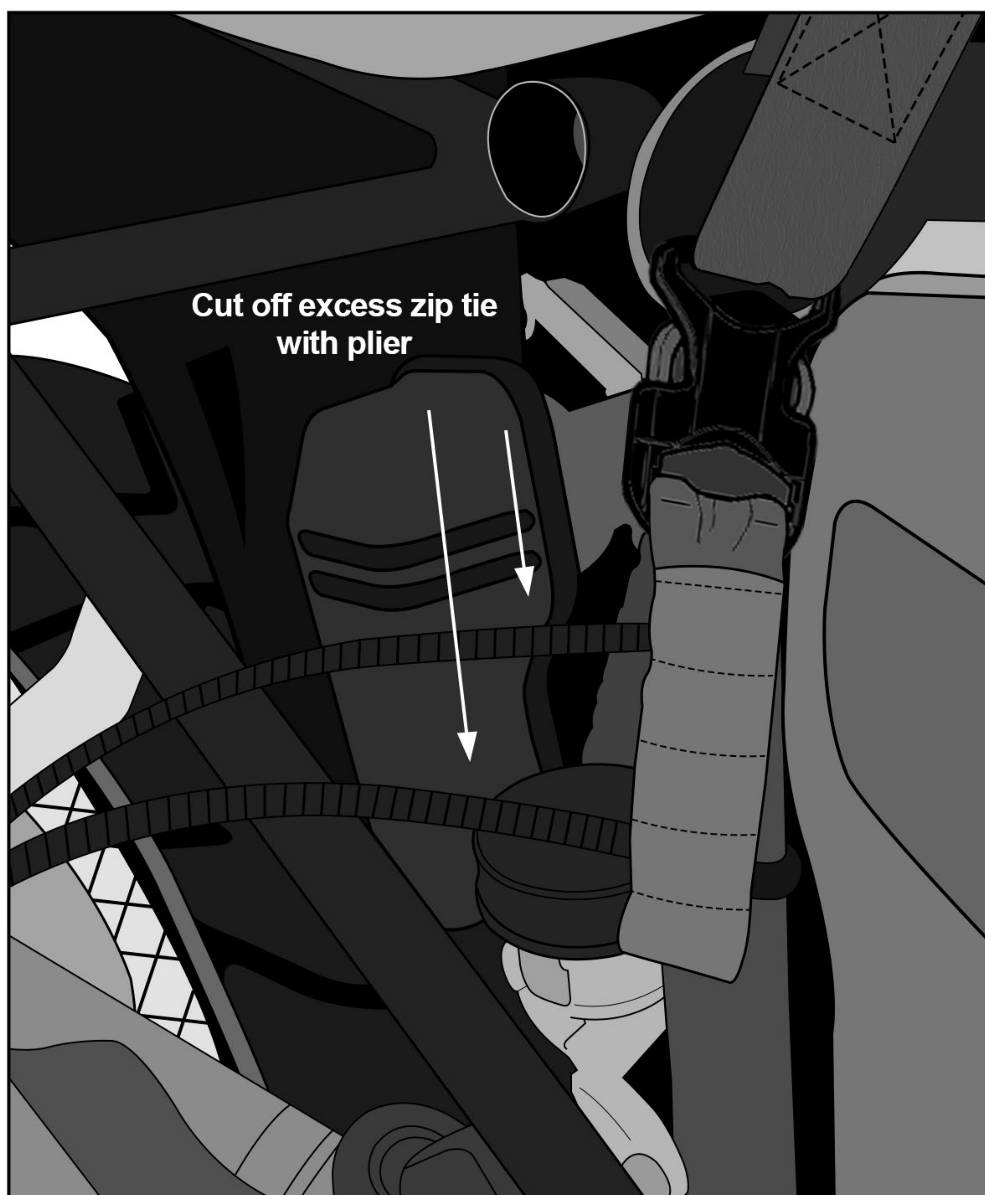
(Fig 4) Once both zip ties are tight and secure, cut off the access zip ties that are hanging
