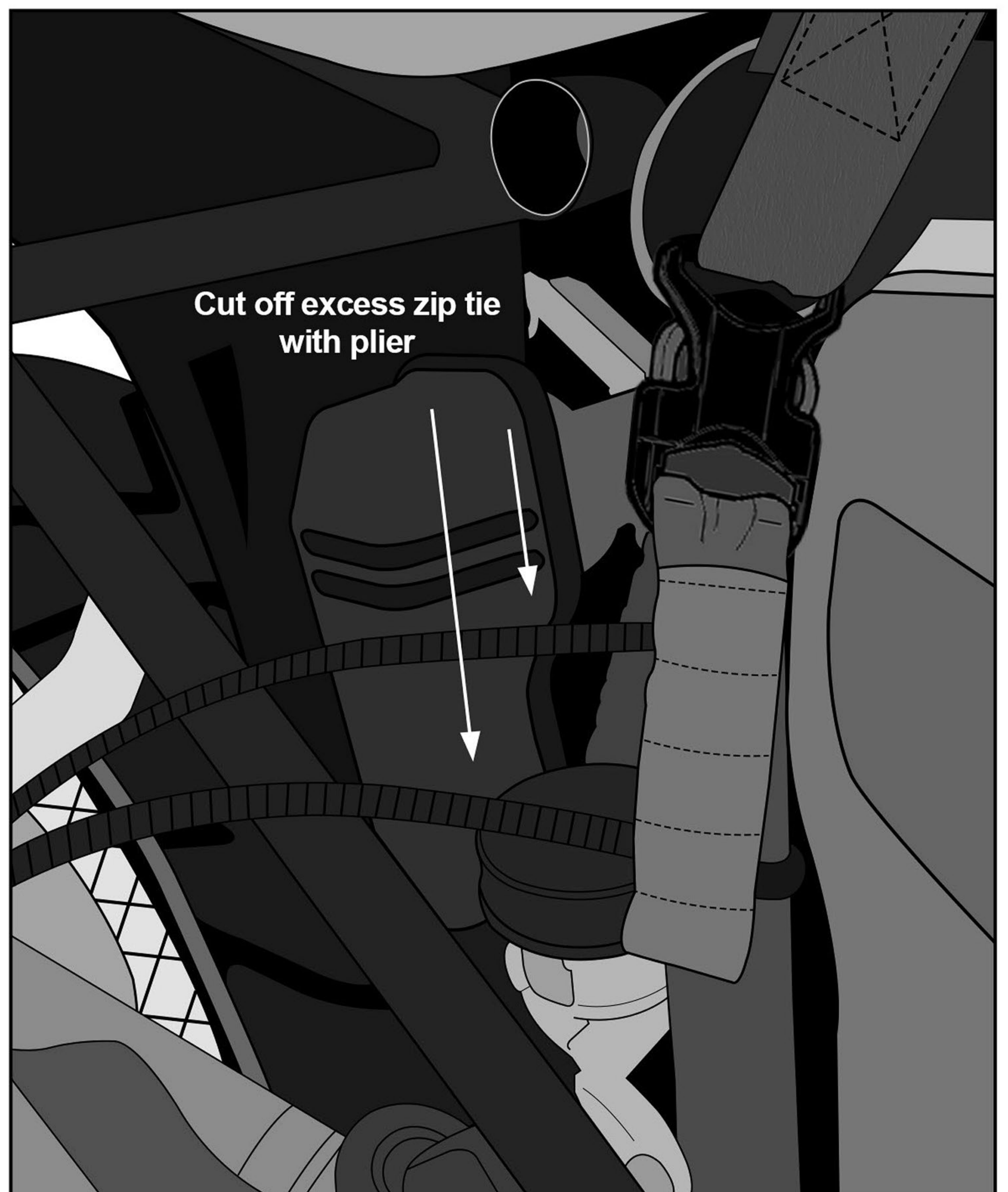
(Fig 4) Once both zip ties are tight and secure, cut off the excess zip ties that are hanging
