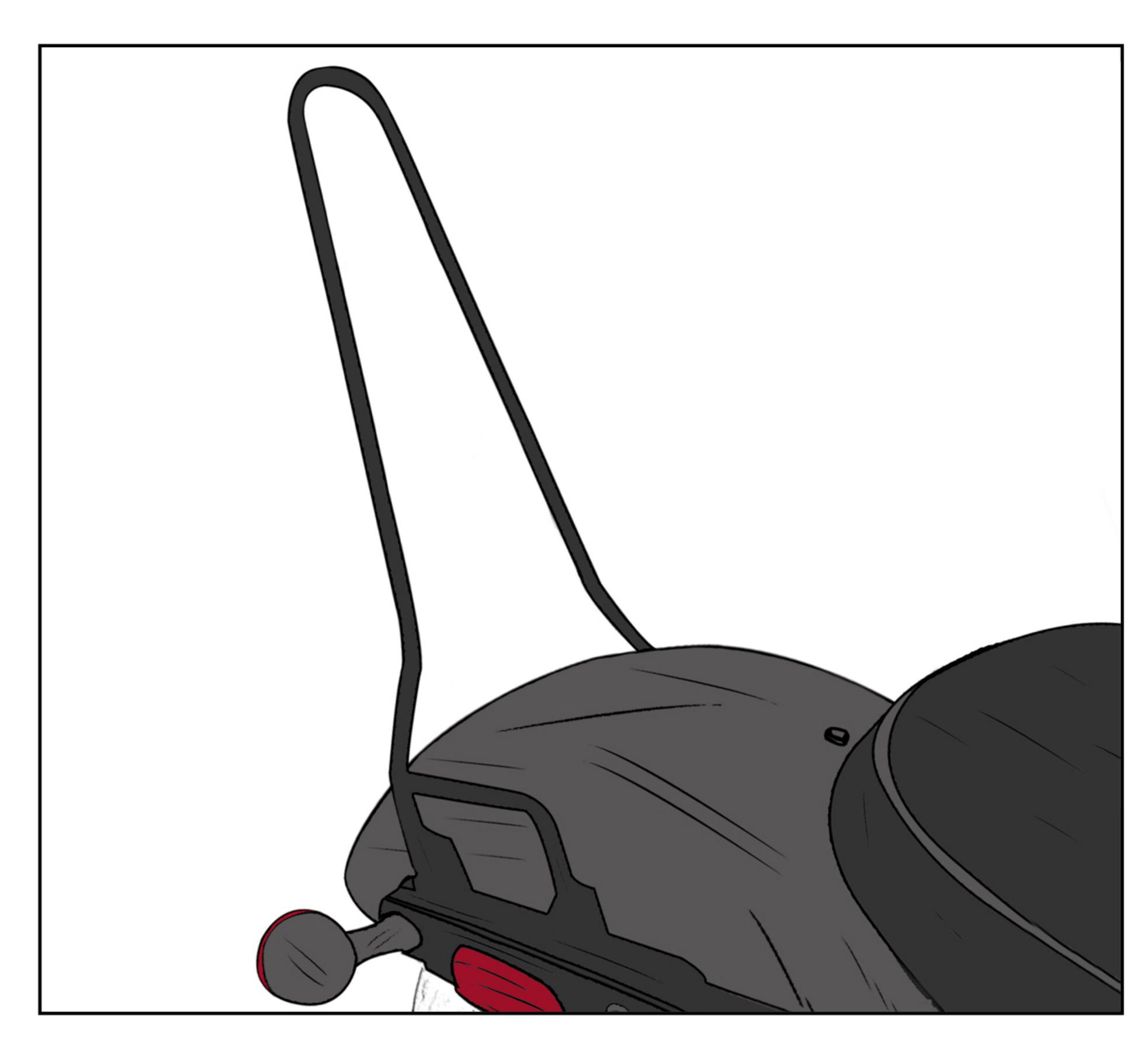
Fig A. Installed between Fender Strut and Rear Fender
