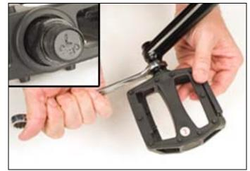
Note: You will damage the threads in the crank arms if you thread the wrong pedal into the wrong crank arm.
