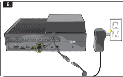
Connect the USB cable to one of the USB ports on the back of the console. Then connect the AC adaptor to the power port on the cable, and the AC to the wall socket.
