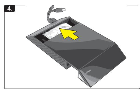
Gently slide on the cover and press into locked position.
