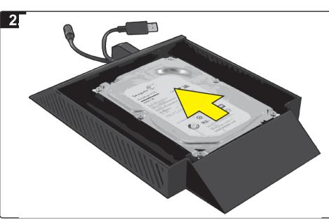
Place the 3.5" hard drive (not included) into the Data Bank and press forward to connect.
