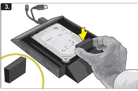
Place the included foam pad between the hard drive and enclosure, to further secure the hard drive from movement.
