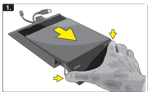
Press and hold the chrome release buttons on both sides of the cover, and gently pull the cover off.
