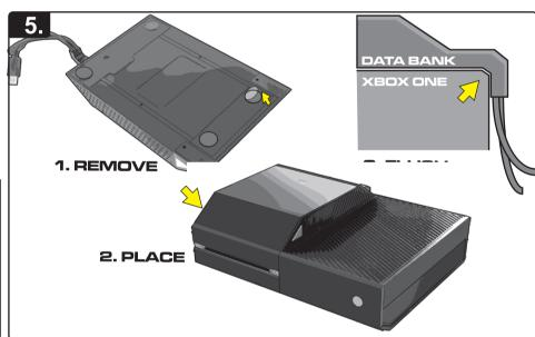
Remove the protective covers from the semi adhesive foam feet on the Data Bank, and place the device on the console surface. Make sure to align the Data Bank on the console properly so that the L shaped cable guide is flush with the back of the console.
