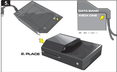
Remove the protective covers from the semi adhesive foam feet on the Data bank, and place the device on the console surface. Make sure to align the Data drive on the console properly so that the L shaped cable guide is flush with the back of the console
