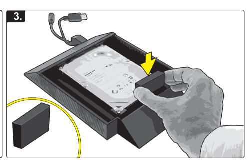
Place the included Foam pad between the Hard Drive and enclosure, to further secure the hard drive from movement
