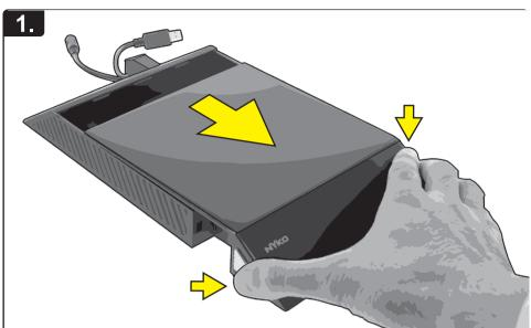
Press and hold the chrome release buttons on both sides of the cover, and gently pull the cover off.
