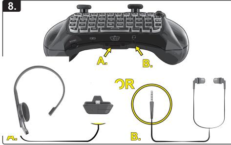
Once properly installed, connect headset (style compatible with your controller) by directly connecting to the appropriate port on the Type Pad.
