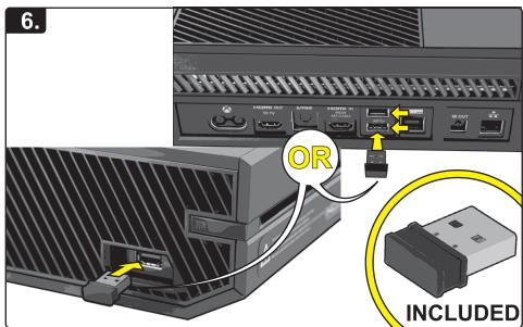
Insert the Wireless Adaptor into an available USB port on the side or back of the console.
