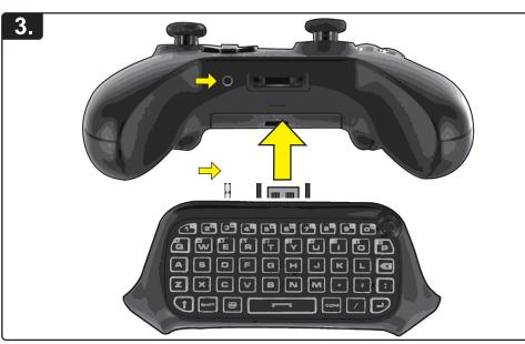
Attach the Type Pad by aligning the plugs and gently pressing into place.
