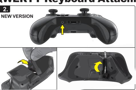
Those with new model XBOX One controllers (with standard headset input) will need to extend the pass-thru headset jack located under the rubber cover on the back of the Type Pad. Gently flip into extended position and replace the rubber cover to cover the storage area.
