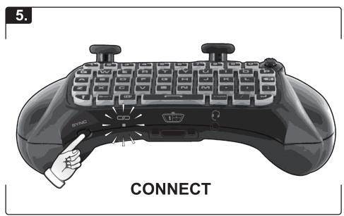
Press and release the SYNC button on the Type Pad to initiate pairing. The LED indicator will blink rapidly to indicate sync discovery mode.
