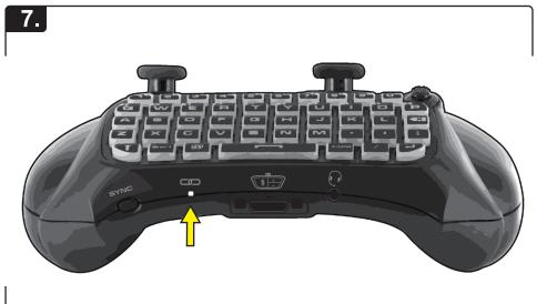
Once properly paired, the LED indicator will glow SOLID blue for 2-3 seconds to indicate successful connection before turning OFF. Test the mini directional pad and buttons to confirm proper operation. Repeat procedure if necessary to establish sync.
