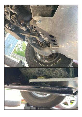
4. Lift the cat protection plate into position. The front of the plate will slide between the front skid plate, and have the aluminum spacers above this. The front bolts slide into the slots on the front, this should help hold the plate up.
