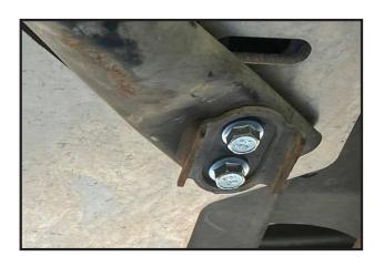
5. Replace the frame to transfer case cross member brace. Use the included hardware to secure the brace to the transfer case cross member. The brace will go on top of the cat plate.
