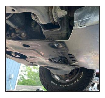
■ 1. Remove the two rear bolts on the OEM front/engine skid plate and allow the rear part of the OEM skid plate to hang down. Reinstall two of the 40mm bolts included with the kit to the skid plate but leave loose. There is an aluminum spacer included that will go on these bolts to space them.
