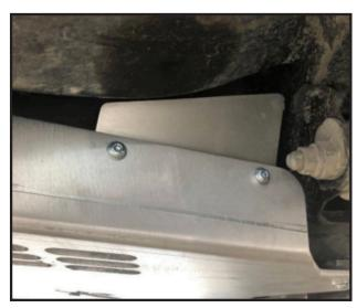
■ 2. Install the winglets on the side of the plate as shown.
