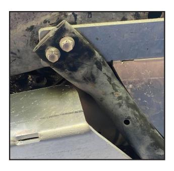
3. Remove the 4 bolts from each brace going from the frame to the transfer case cross member. Remove both braces and set to the side.
