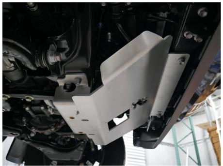
3. Install front skid plate on truck. The front holes will be the same as the factory braces. Reuse bolts from the factory front skid plates braces to install front plate to radiator cross member on truck. The rear portion will use 2 M12x30 mm Allen bolts to mount to the bracket.
