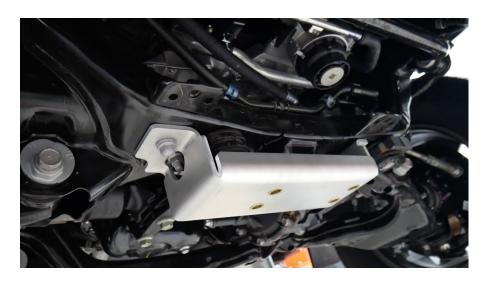
2. Install front skid plate bracket in rear holes from factory front skid plate braces. Reuse factory bolts. Leave bracket loose to allow for adjustment later.
