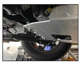
■ 3. The front felt bracket may be removed or left in place. If keeping the engine felt liners you will need to leave it in place. Loosen the M10x1.5 Bolts so there is approximately a ½" gap. You will slide the front slots of the transmission skid plate onto these bolts. If the factory felt liner bracket is left in place, we recommend removing the spring clips to prevent a rattle. We are now including M10 button head bolts which can be installed instead of the M10 hex bolts if desired.
