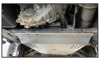
■ 5. Locate the 3/8-16 3.5" long bolts with washers and nylon lock nuts. These will go into the slots on the frame and a washer and nut will attach at the top. The slot may have an adhesive heat shield on it, and this will need to be penetrated prior to pushing the bolt through it. Shown above is the driver side. If you have an FX4 transfer case skid it will need to go above the transmission plate.
