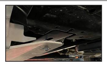
4. Slide the front of the transmission skid plate onto the front bolts. The factory felt liner bracket will go above the transmission skid plate, in between the transmission skid plate and frame. If you have a factory FX4 Skid plate this will go above the transmission skid plate, between the skid plate and frame.
