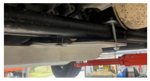
■ 5. Install 2-3/8 4" long bolts, 1.5" fender washers and transfer case backing plate around frame at rear of transfer case. Use 2 3/8 nylon lock nuts on top of plate.
