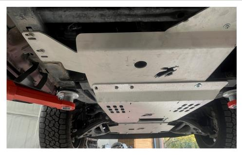
■ 4. Slide transfer case plate in between transmission plate and truck frame. Install two M8x40mm bolts on driver side frame into nut plate.
