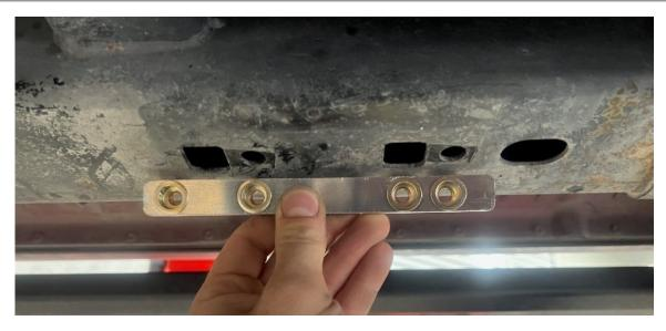
Inset driver side nut plate into frame. Alternatively, OEM spring nuts can be used if OEM skid plate was installed. One set of holes are for the F-150 Non-Hybrid and the other is for the Hybrid Powerboost models.
