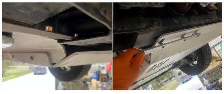
Insert passenger side nut plate into frame. It may be necessary to insert it from the hole in the middle of the frame that gives access to the rear transmission mounts. Loosely install three M8x40mm allen head bolts with 3/8-1" washers into nut plate.
